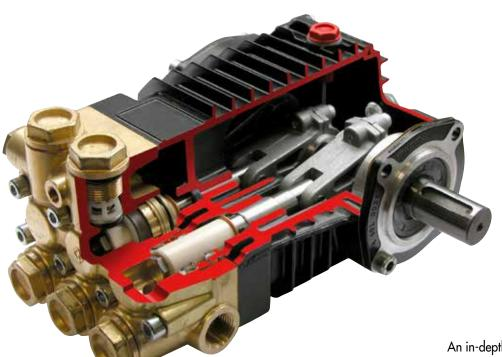
An in-depth and comparative study on each structural element: • Low wear and tear ceramic pistons • Low friction connecting rod, built in aluminium alloy; double body for easy disassembly • Minimum charge on the cone-shaped bearings (through electronic calibration of the drive shaft rotation) • Very low operating temperature, favored by the use of water cooled motor • Top range up to 21 l/min.
