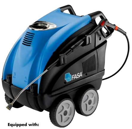
4 poles electrical motor (1450 RPM) with thermal protection and water cooling (three phase models) • Three ceramic coated pistons, brass linear pump head (1 ph), full ceramic pistons (3 ph), brass linear pump head with built-in by-pass valve • Vertical burner with high thermal efficiency steel coil.
