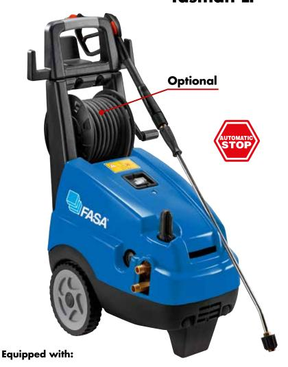
• 4 poles electrical motor (1450 RPM) with thermal protection and water cooling • Three ceramic coated pistons,(full ceramic pistonsonly for Tasman 1713) brass linear pump head with built-in by-pass valve. • Suction and delivery S. S. valves. • Low voltage and delayed Total Stop (three phase models) • Detergent tank (2,8 lt.). • Pressure regulator. • Glicerine pressure gauge. • Hose-reel (on request)
