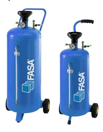
**Spray:** Pneumatic charge sprayers need to be connected to an air compressor to charge the tank and allow the product vaporization without the connection to the air compressor. They work at high-pressures and so they use capacious steel or stainless steel tanks to allow a greater working autonomy.
