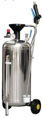
Continuous pneumatic foam sprayers need a permanent connection to an air compressor; in this way air mixes with the chemical product producing a soft and voluminous foam that persists on surfaces: with a little chemical product, it is possible to treat wider areas or tough dirt (also on ceilings, inclined and/or slippery walls). They work at high-pressure and so they use capacious steel or stainless steel tanks to allow a greater working autonomy.
